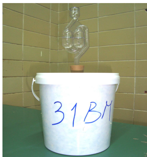
Figure 1. Mini-silo for silage study
